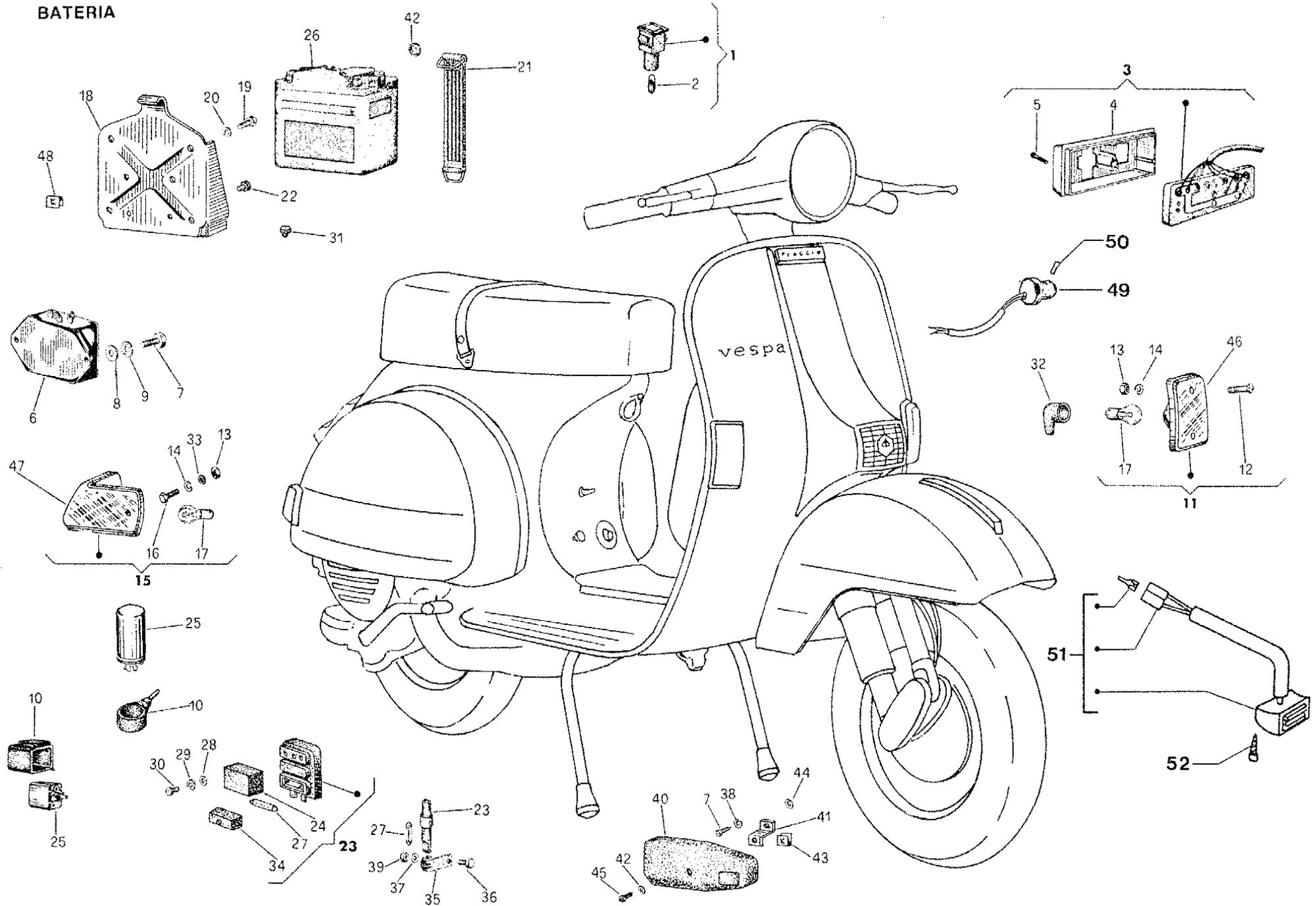
DISPOSITIVI ELETTRICI (VEICOLI CON AVVIAMENTO ELETTRICO) — DISPOSITIF ELECTRIQUES (VEHICULES AVEC DEMARRE ELECTRIQUE) — ELECTRICAL DEVICES (VEHICLES WITH ELECTRICAL STARTER) — ELEKTRISCHE AUSRÜSTUNG (FAHRZEU MIT ELEKTRISCHEN ANLAßER) — DISPOSITIVOS ELECTRICOS (VEHICULOS CON ARRANQUE ELECTRICO)
