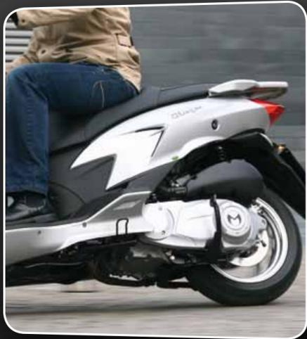
BLOG is equipped with an the innovative and reliable 160 or 125 cc, liquid cooled, electronic injected engines, which grant excellent results in terms of performance and driveability under any condition. The 4-stroke engines are the outcome of an important international project about the electronic injection. They assure pollutant emissions even lower than the EURO 3 standards.
