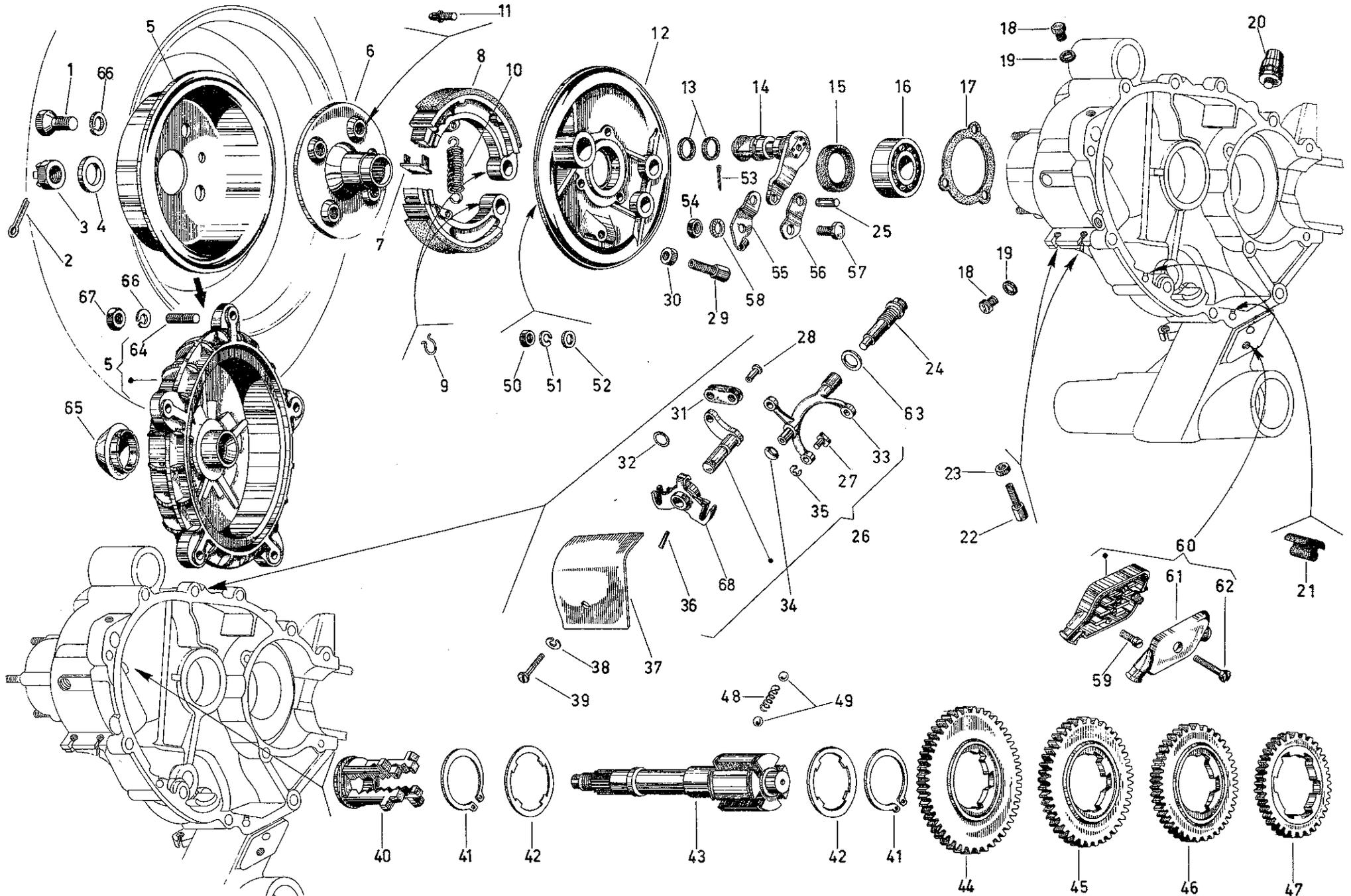
T. IV VOLANO - BOBINE — VOLANT - BOBINES — FLYWHEEL MAGNETO - COILS — VOLANTE MAGNETICO - BOBINAS
