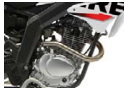
Motor 4T 2V refrigerado por aire Euro3/Motore 4T, 2V, raffreddato ad aria Euro3/4-stroke, 2V, air cooled engine Euro3.
